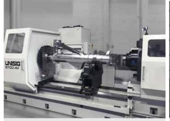
UNISIG B700 BTA machine with drop bed to swing up to 63 in [1600 mm] for commercial landing gear
