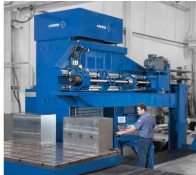
**USC-TS Deep Hole Drilling Machines** For Drilling Heat Exchanger Tube Sheets
