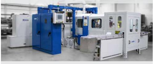
High-accuracy gundrilling of small parts with multiple off-center and angled holes from 0.8 mm to 6 mm [0.03 to 0.25 inch] diameter up to 150 mm [6.0 inch] deep.
