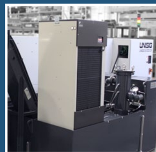
COOLANT REFRIGERANT CHILLER Upgrade from heat exchanger for precise temperature control regardless of ambient temperature.
