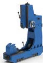
**Lantern chucks** allow a pull boring tool to be easily installed and aligned during the drilling process, without requiring a special pilot hole machined in the part.
