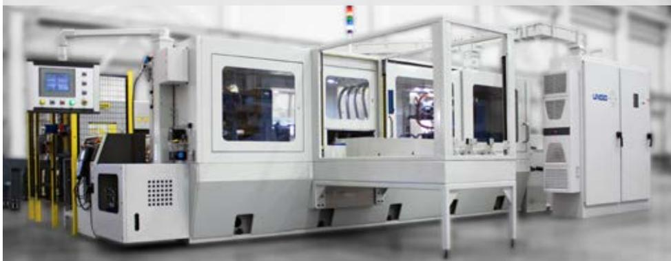
Powerful four-spindle machine for production BTA drilling of holes from 12 mm to 25 mm [0.47 to 1.0 inch] diameter up to 750 mm [30 inch] deep.
