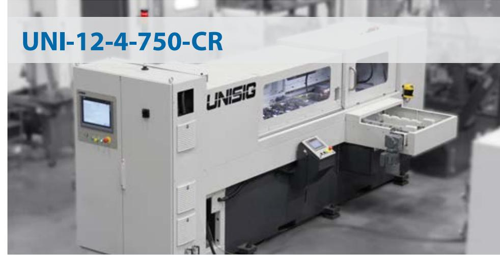
High-volume production gundrilling of shafts with very straight holes from 3 mm to 12 mm [0.12 to 0.50 inch] diameter up to 750 mm [30 inch] deep.
