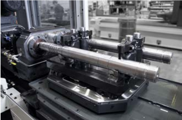
CNC positioning, rotary motion and modular workholding are available for complex drilling operations in production
