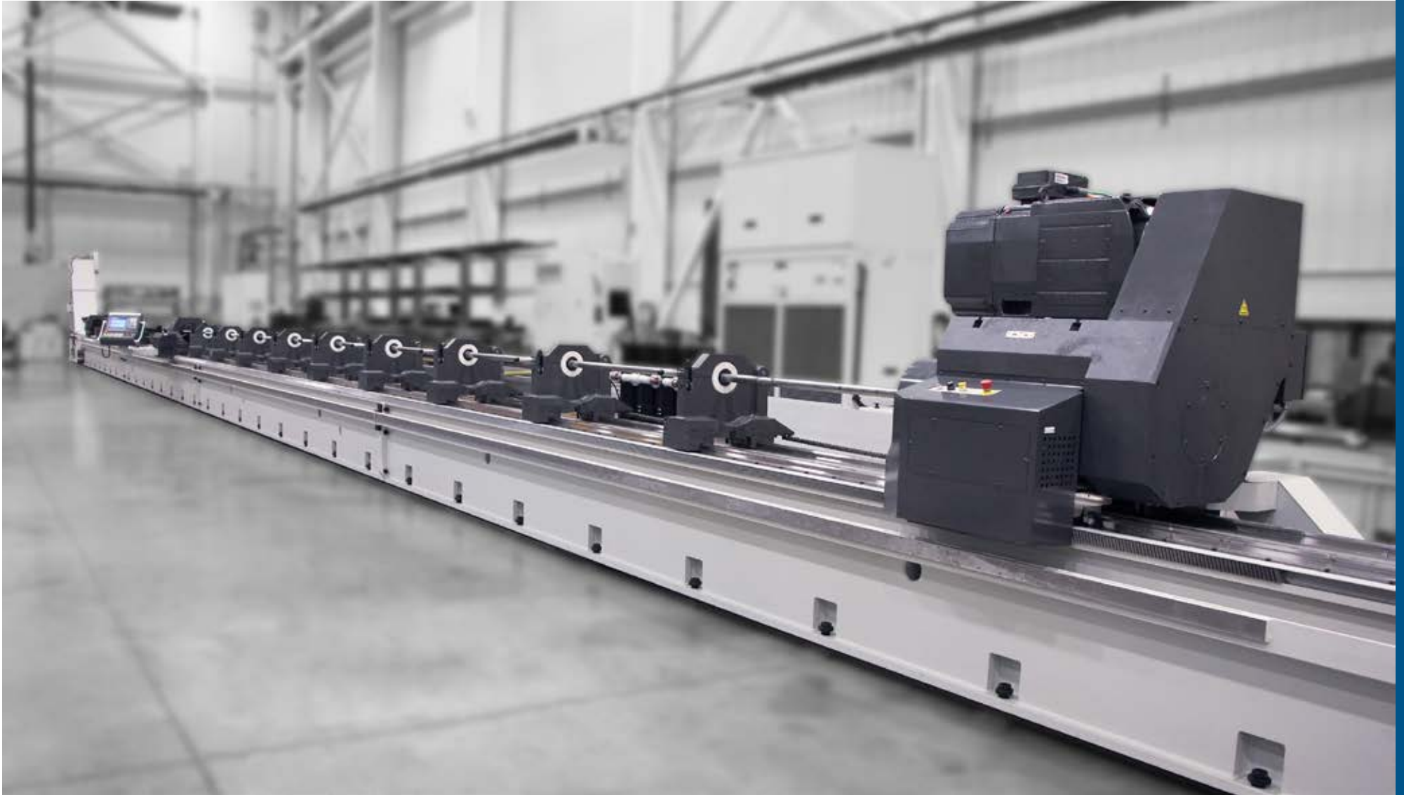
UNISIG S-Series skiving and roller burnishing machine, used to produce precision bores up to 42 ft [13 meters] deep
