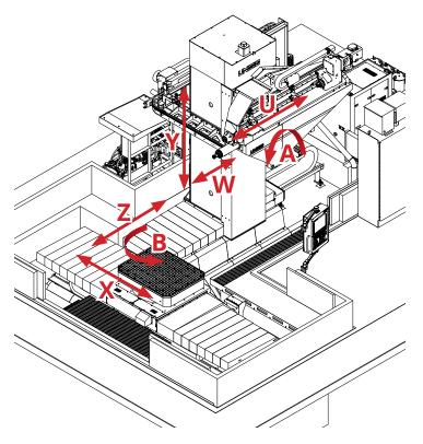
7-axis machine - **X Y Z W U** linear axes + **B**-axis rotary table + **A**-axis inclining headstock
