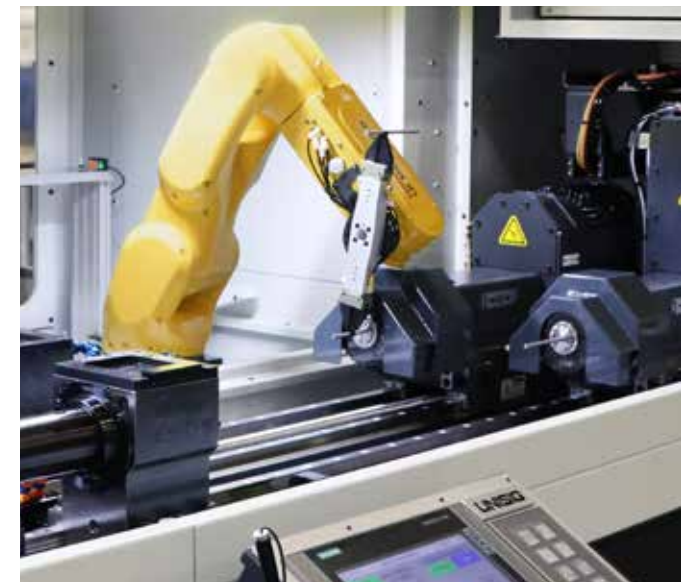
UNE6 configurations offer single-spindle, or two independent spindle layouts, with optional robot ready or robotic automation.
